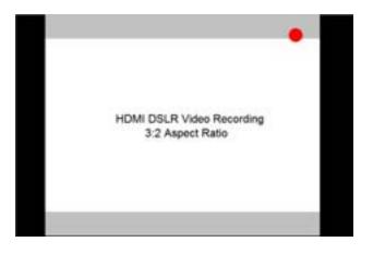
Use the **16:9** option to scale the HDMI DSLR video output to fit the 16:9 portion of the screen. This will also remove the portion of the on screen video that is NOT recorded by the DSLR camera due to sensor crop.
