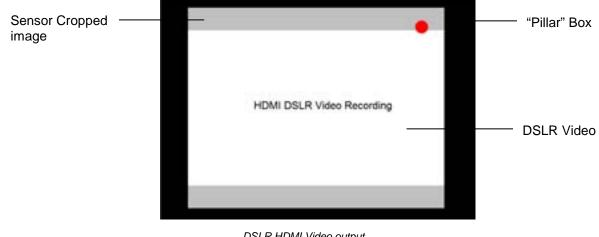
DSLR HDMI Video output during recording
