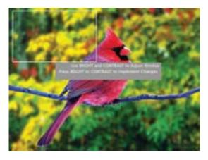
2. Using the BRIGHT and CONTRAST knobs, select the portion of the image you would like to view with scaling turned off. The BRIGHT knob will move your selected area left and right, and the CONTRAST knob will move your selected area up and down.
