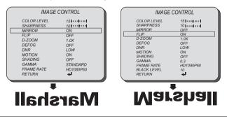
Select IMAGE CONTROL using the UP or DOWN button. You can select D-ZOOM, DEFOG, and DNR using the UP or DOWN button.
