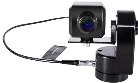
The **CV-PT-HEAD (µL)** can be controlled by CV-MICRO-JYSTK or any BR Remote style controller. These controllers generate RS485 data which can be connected directly to the CV-PT-HEAD or sent via an IP network with IP adaptors. The RS485 data can be sent up to 3,000+ feet (1km) on a four (4) pin XLR cable.
