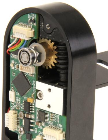
The tilt clutch adjuster is accessed by removing the Main Cover. This has 3 screws. Take care not to damage the sealing gasket. The Tilt Shaft Support Bearing may be on the shaft, as in this picture, or may be retained in the main cover. Take care not to lose this bearing.
