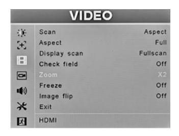
This page provides controls for picture size, position and related functions including image flip, image freeze and Zoom.
