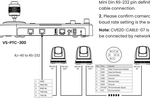
1. Please refer to the RJ-45 to RS-232 and camera Mini Din RS-232 pin definitions to complete the
