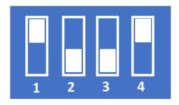
In this example, audio incoming from HDMI be sent to the HDMI and USB outputs. The audio from the Analog inputs will be sent to the Analog output only.
